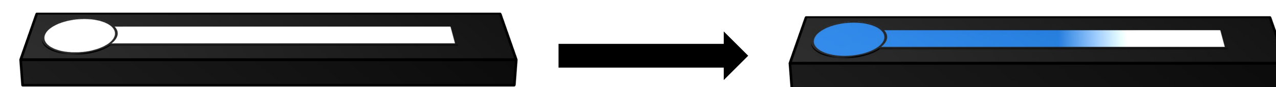
Figure 1: A schematic of a \mu PAD, producing a response to a microvolume of water.
