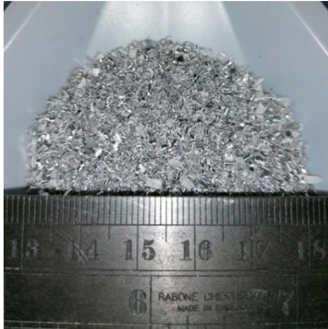
Figure 3.1 WE43C scraps produced from the machining
