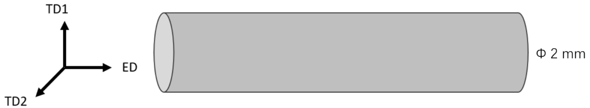
Figure 3.6 A schematic of coordinates for SS-FSC extruded (CoreFlowed) wire
