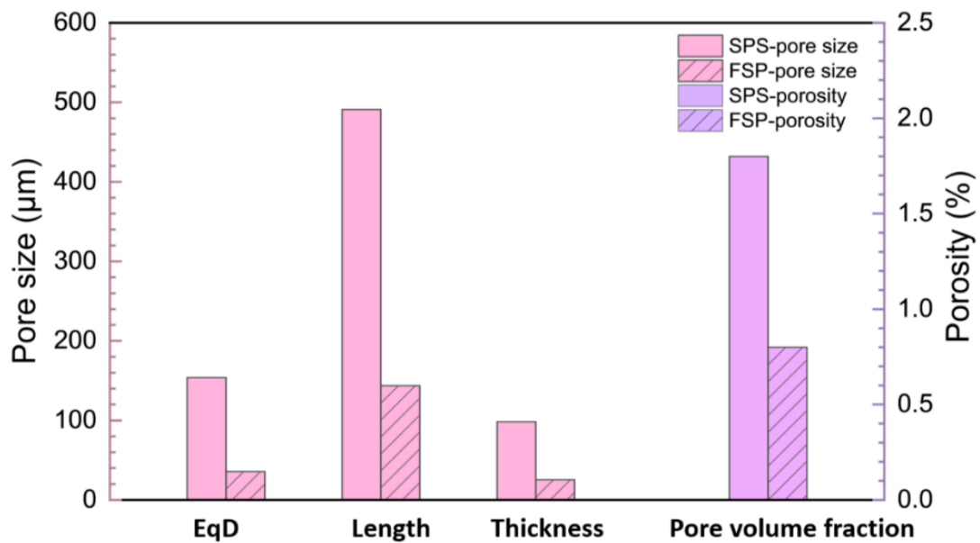
Figure 6.5 The comparison regarding pores in the SPSed and FSPed material
