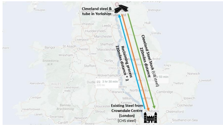
Figure 4. Transferring steel from Crowndale Centre to Cleveland Steel (Yorkshire) for the reclaiming process (Author)
