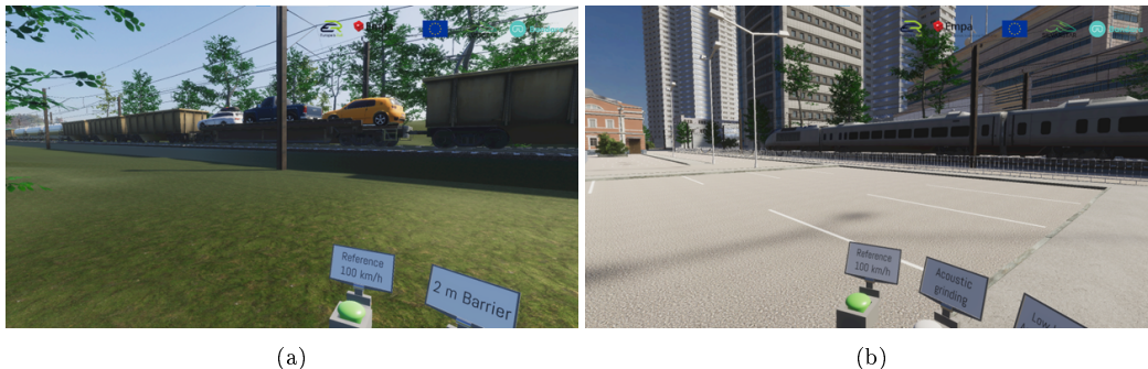
Figure 2: Examples of the user view of the SILVARSTAR VR demonstrator with train passages in different environments and the virtual buttons (bottom right) for activating different mitigation measures in real time. (a) Freight train in rural setting. (b) Intercity train in urban setting.
