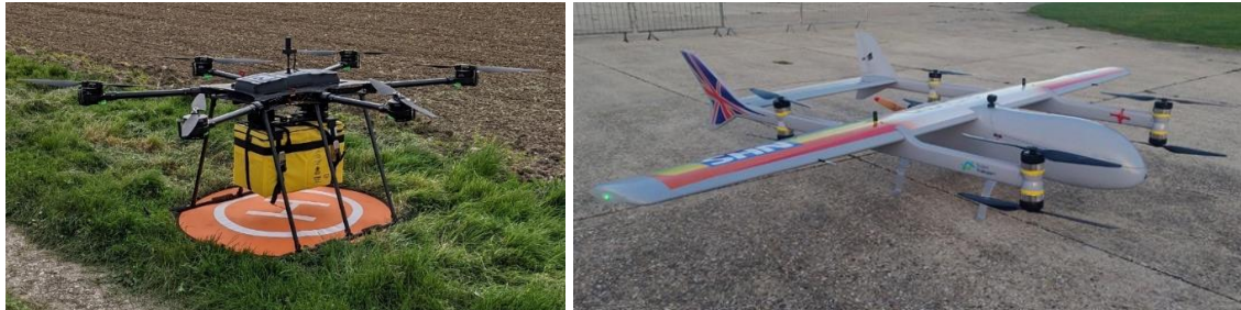
Figure 2. Multi-copter drone platform (left) and VTOL/FW hybrid drone platform (right). Both drones are shown loaded with one medical container (dimensions 460×255×305 mm, Figure 3), which is underslung for the multi-copter drone and contained within the cargo compartment located in the forward fuselage for the VTOL/FW hybrid drone (wingspan of ~5 m).
