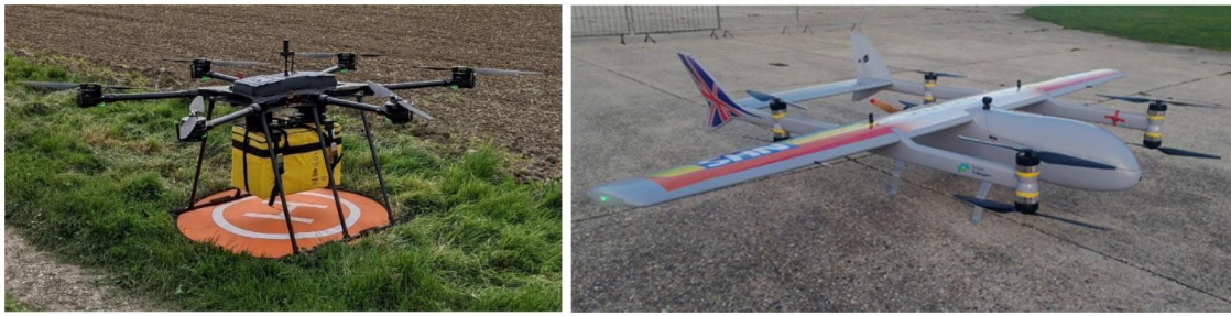
Figure 2. Multi-copter drone platform (left) and VTOL/FW hybrid drone platform (right). Both drones are shown loaded with one medical container (dimensions 460 \times 255 \times 305 mm, Figure 3), which is underslung for the multi-copter drone and contained within the cargo compartment located in the forward fuselage for the VTOL/FW hybrid drone (wingspan of \sim 5 m).
