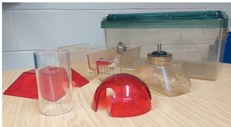
Figure 1. Objects used to house laboratory mice. From right to left: standard individually ventilated cage for mouse; water bottle; enrichment dome (translucent red); food hopper; enrichment fort (translucent red); mouse handling tube.
