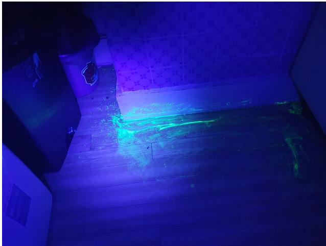
Figure 6. Despite cleaning, the dust remains visible under the black light. Credit: Author.
