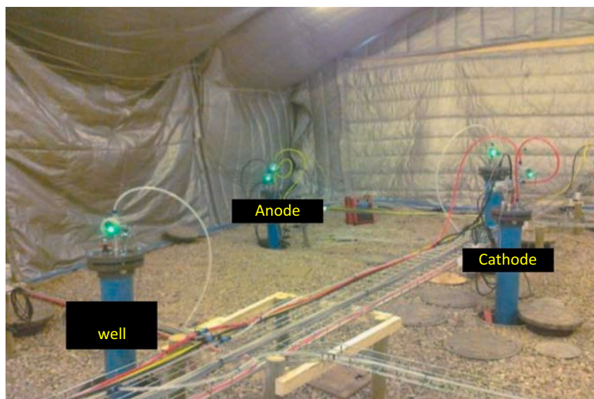
Fig. 20. Example of the EKR-Bio trial (2018) undertaken on tetrachloroethylene-contaminated soil in Denmark. Lactate and sodium hydroxide additives were used to stimulate bacterial growth (Riis et al., 2012).
