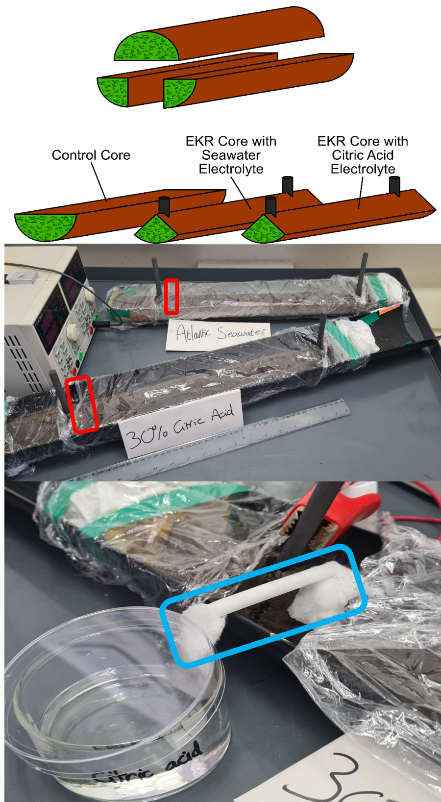
Figure 5.3 – Top - schematic showing how the collected core was divided up. Grey bars represent the location of graphite electrodes. Middle – photo of the experimental setup, with the locations of the electrolyte ‘bridges’ were placed marked in red. Bottom – photo of the citric acid core electrolyte ‘bridge’ (marked in blue). The system functioned by allowing electrolyte to move by capillary action from the reservoir, through the cotton wool, and onto the core. A transparent plastic tube was put around most of the cotton wool to minimise electrolyte evaporation and contamination.
