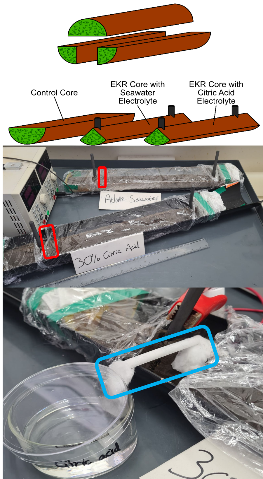
Figure 6.3 – Top – schematic of the divided sediment core, with the grey bars indicating the position of the electrodes. Middle – photo of the experimental setup, with the positions of the electrolyte ‘bridges’ indicated in red. Bottom – photo of the citric acid core electrolyte ‘bridge’ (highlighted in blue). The system operated by drawing electrolyte from the reservoir, through the cotton wool, and onto the core. To reduce evaporation and contamination, the majority of cotton wool was enclosed within a transparent plastic tube.
