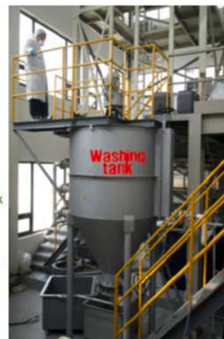
Fig. 5. Schematic of the set-up used by Kim et al. (2015a) on the 800 L scale EKR process on contaminated KAERI material, with washing drum highlighted on the right. The drum is several metres tall so is a significant improvement from laboratory scale.
