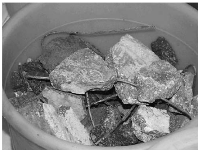
Fig. 6. Examples of the concrete examined by Yurchenko et al. (2009) complete with reinforced steel pins used in construction. X-ray (Rietveld) analysis indicated \alpha -quartz, orthoclase and plagioclase feldspar, calcite and boltwoodite – \text{H}(\text{K},\text{Na})(\text{UO}_2)(\text{SiO}_4) \cdot 1.5(\text{H}_2\text{O}) – phases in the concretes.
