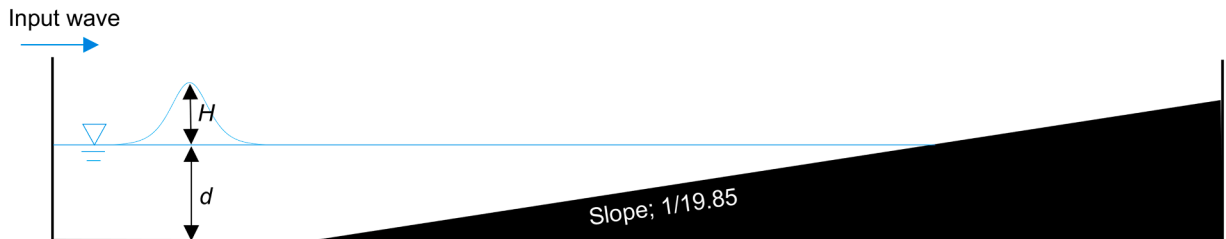
Fig. 3. A schematic diagram of a laboratory experiment by Synolakis (1987).
