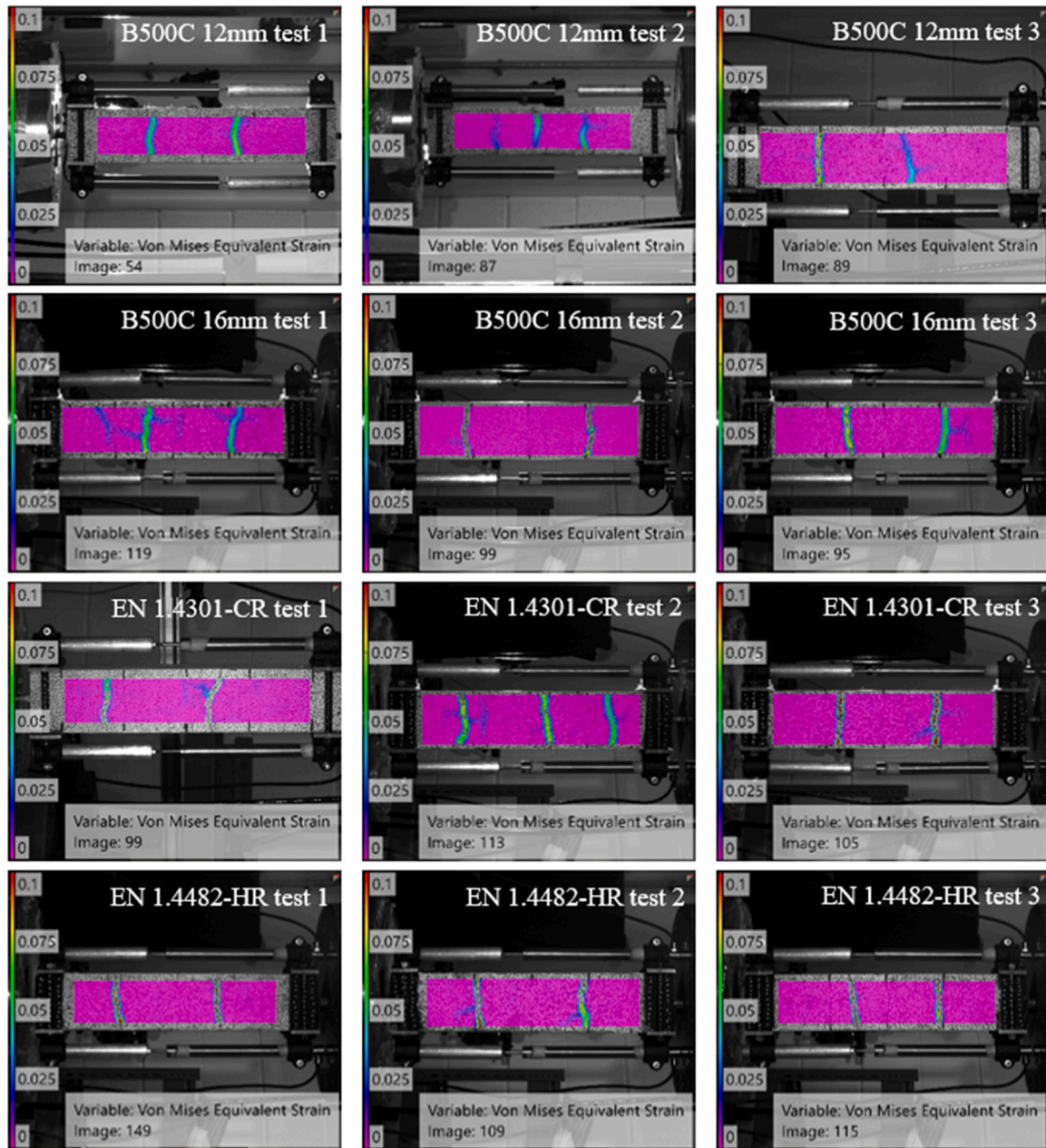
Fig. 9. DIC images of crack patterns of tension stiffening responses at rebar yield stress.
