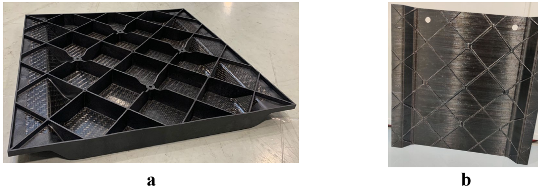
Figure 1 – a) overmoulded organosheet panel; b) organosheet panel with no ribs (no injection)
