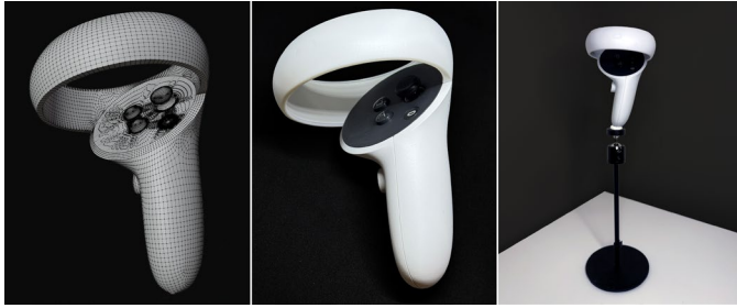
Fig. 1. Meta Quest 2 right controller – The digital reference model (left), the physical controller used in the scans (center), and the scanning setup (right).
