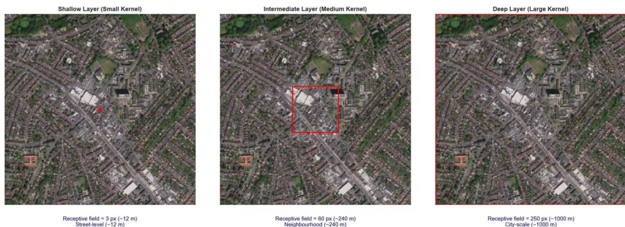
Figure 3.6 Conceptual illustration of receptive field expansion in CNNs
