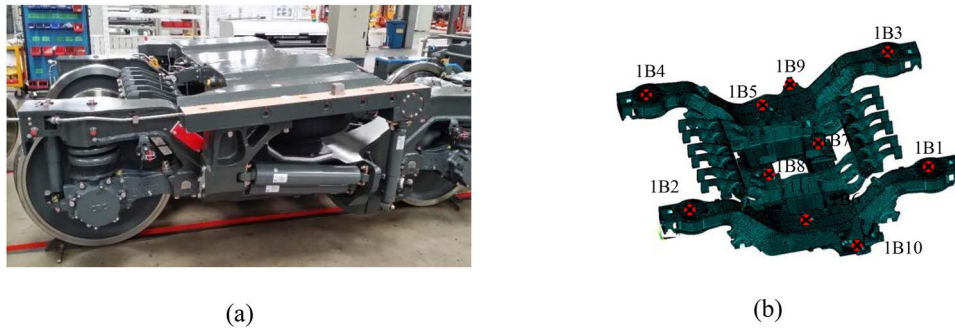
Figure 20. The bogie, bogie frame, and measurement points. (a) A photo of the bogie; (b) the layout of measurement points on the bogie frame.
