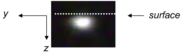
Figure 4.9: Nomenclature of mode profiles used in this thesis with the z direction specifying the crystal depth and y direction the spatial direction equivalent to across the beam. The white dashed line is the crystal surface.
