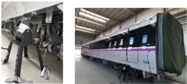
Fig. 1. The measured vehicle body and exciter
