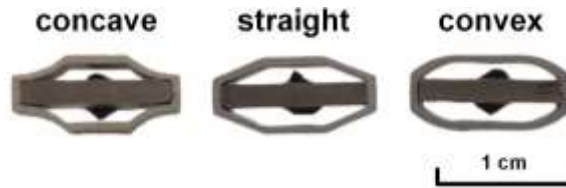
Fig. 2 Prototypes of the class IV miniature FTs incorporating concave, straight, and convex metal shells, respectively.
