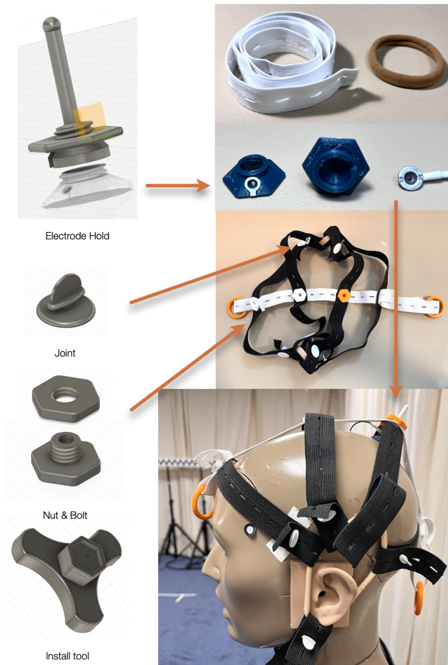
Figure. 11.7. Design and assembly of the self-constructed EEG cap
