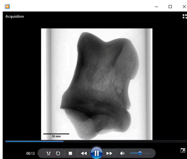
Fig. 8. Still image captured from Supplementary Information Video 2 . 360-degree radiographic inspection of the phalanx. The radiographs were captured during the \mu CT acquisition process and serve as the basis for reconstructing the volumetric image.
