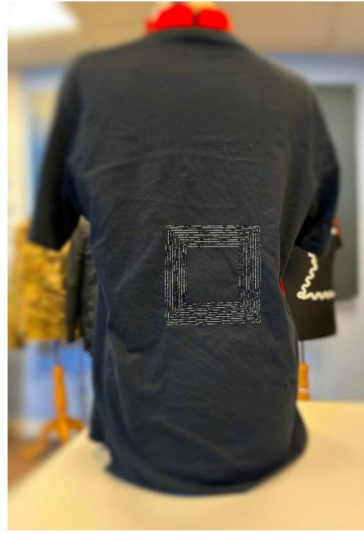
Fig. 9. Example coil on a t-shirt used in wash testing.
