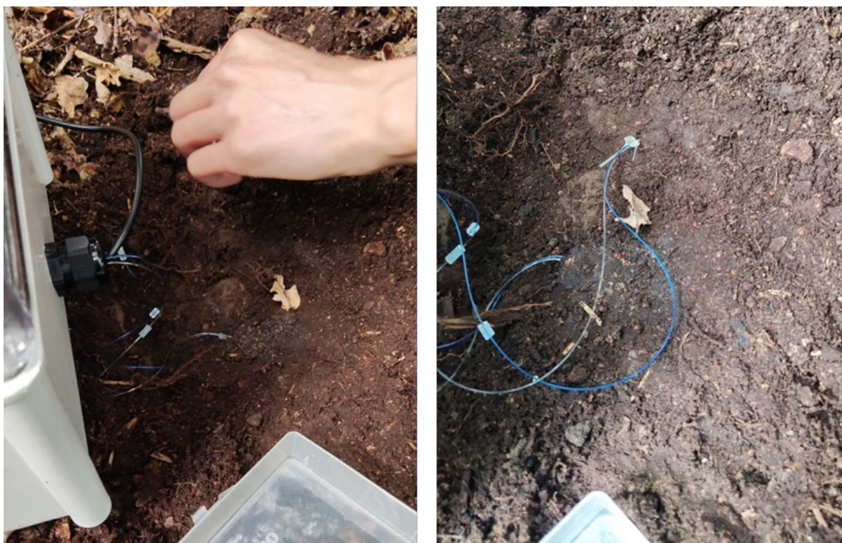
Figure 34 Installation of the microdialysis probes into the soil at Writtle using the two different methods.
