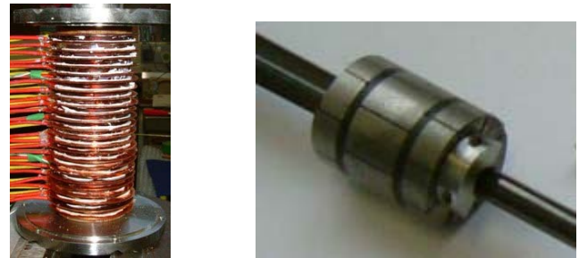
Figure 2: Photographs of the stator (left) and the PM shuttle and shaft (right).
