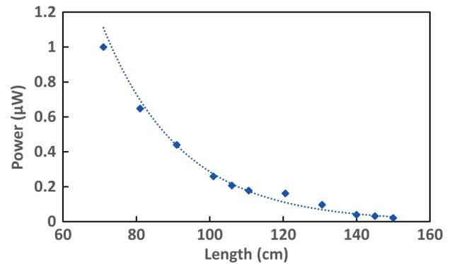
**Fig. 7.** Example cutback measurement of integrated power over 700 nm to 1800 nm of a 5- $\mu\text{m}$ -diameter silicon core fiber drawn at  $10 \text{ m min}^{-1}$ . The light source was a Fianium WhiteLase SC480. Blue dashed line is an exponential fit corresponding to a loss of  $0.2 \text{ dB cm}^{-1}$ .
