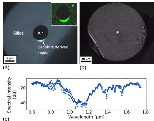
**Fig. 8.** (a) Bottom lit micrograph of a cleaved end of initial sapphire ( $\text{Al}_2\text{O}_3$ ) derived core fiber fabrication test. The draw was a test of material compatibility between sapphire derived core (bright crescent) and the silica capillary. The inset shows the EDS map of aluminum in the central region of the fiber. (b) Micrograph of silica fiber with a Ti-doped core drawn from a preform prepared using glass powder deposition. (c) Transmission spectra of the Ti-doped fiber.
