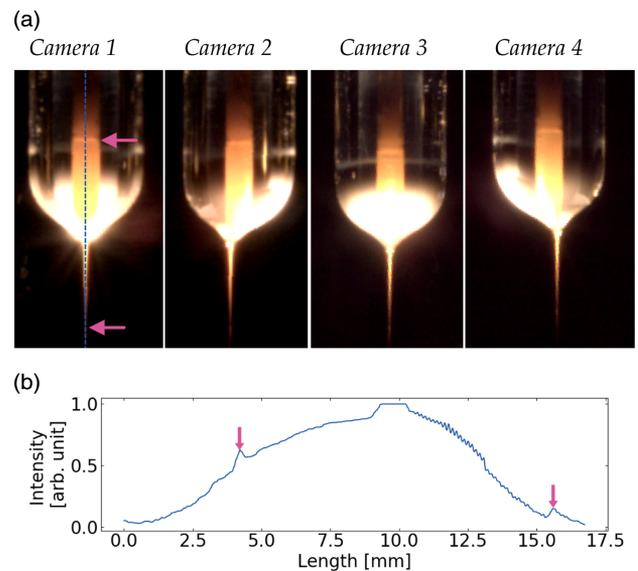
**Fig. 5.** (a) Example image of the hot-zone region in the draw tower furnace during fiber fabrication. Preform is constituted of a silicon core and silica cladding. Camera placement in the furnace is shown in Fig. 2. (b) Intensity profile measured along the blue dashed line in Camera 1. The peaks in intensity (indicated by pink arrows) show the boundaries of the silicon melt zone.
