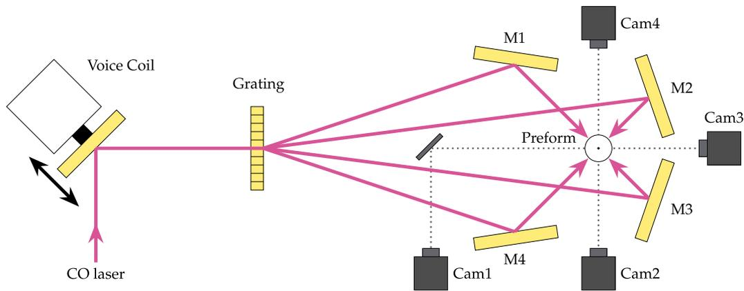
**Fig. 2.** Top-view schematic of the tower furnace design. The CO laser beam was incident on a gold mirror mounted onto a voice coil. The voice coil was driven by a function generator for the controlled oscillation of the mirror. The CO laser beam was split into four by the grating. All beams were in the horizontal plane. Mirrors (M1–M4) directed the beams onto the preform. The hot-zone was monitored by cameras at orthogonal angles (Cam1–Cam4).
