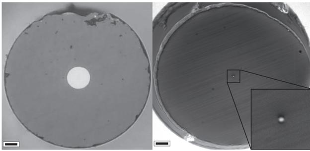
**Fig. 6.** Polished ends of silicon core optical fibers. (left) 20- $\mu\text{m}$ -diameter core fiber. (right) 1.3- $\mu\text{m}$ -diameter core. Black scale bar is 10  $\mu\text{m}$ .
