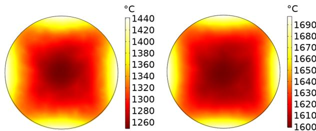
**Fig. 4.** Simulated transverse temperature gradient in the hotspot of the 6-mm-diameter preform after 11 s (left) and 60 s (right) of CO laser exposure. These times correspond to the temperature response shown in Fig. 3.
