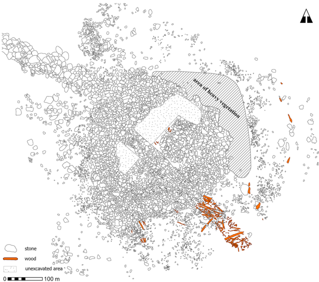
Figure 6. Plan view of stone and timber elements above and below the waterline, digitized from multiple integrated photogrammetry survey datasets.
