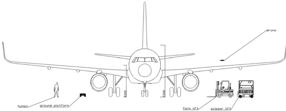
Figure 4. The front view of relevant assets inside a hangar in real scale (aircraft Airbus A320).
