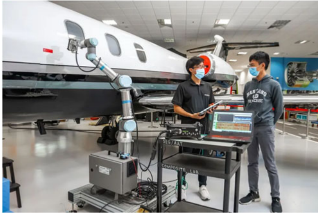
Figure 8. Ultrasonic inspection using a cobot on a static base. Credits: Universal Robots and Olympus [48].
