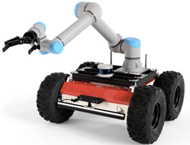
Figure 9. Panther platform can support a cobot and add mobility to the inspection. Credits: Husarion [49].
