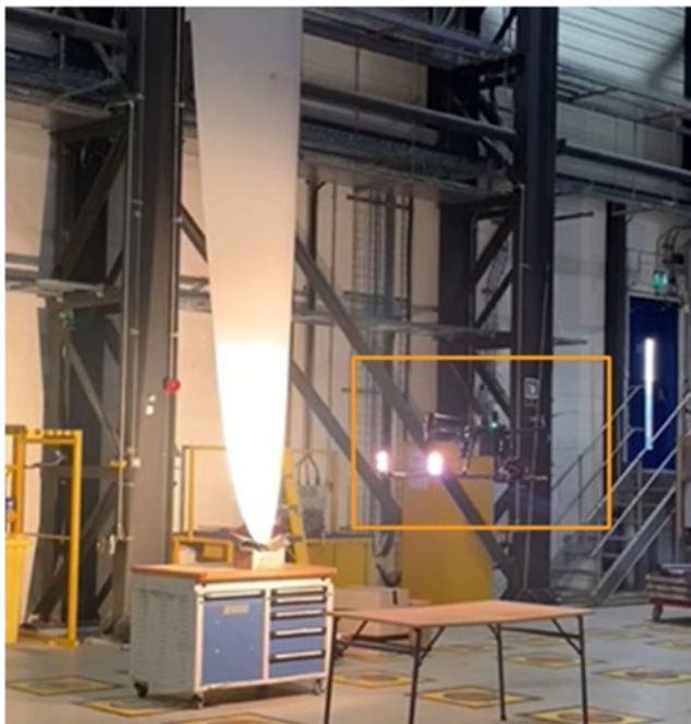
Figure 7. Active thermography UAV experiment on wind turbine blade (composite structure). Credit: Deane et al. [46] (CC-BY).
