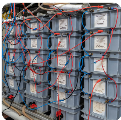
B MFC system receiving urine and greywater
