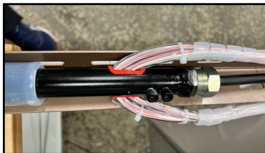
Figure 5: Cable top connection with the load cell, using a stiffener arrangement
