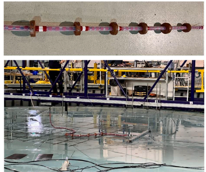
Fig. 4. Cable with buoyancy modules (top) and its arrangement in the FloWave test facility (bottom). When the tank floor is lowered, the cable profile becomes a lazy wave.
