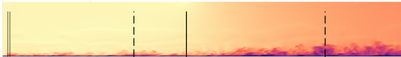
FIGURE 5.2: Side view of the computational domain for the APG flat plate with: trip strip ( 10 \leq x \leq 14 ); recycling plane ( x = 250 ); pressure gradient application location ( x = 350 ); and sampling plane for statistics ( x = 614 ) marked.
