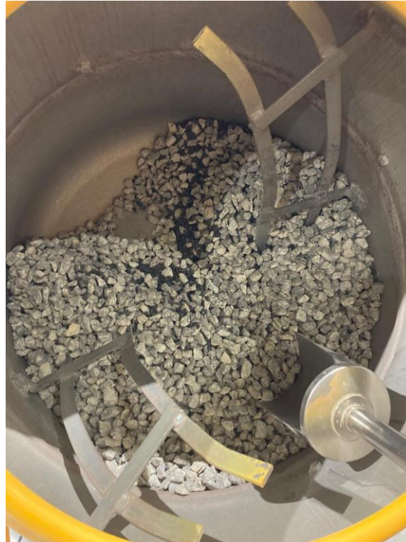
Figure 6. Core of crumb rubber particles after using cement mixer.
