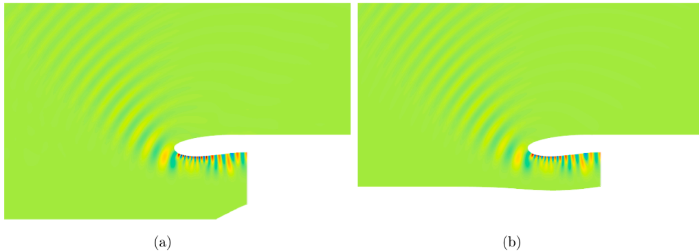
Fig. 19. Pressure field in the FE domain for the rotor-locked m = 22 mode calculated in ACTRAN for both full and part-span ( \nu = 0.5 ) domains. (a) Full domain. (b) Part-span domain ( \nu = 0.5 ).
