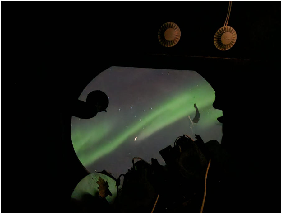
Figure 3.2: HiTIES view out of the dome at the KHO, taken by me in January 2025. SIF is visible in the lower right hand side of the image where the two freshly added ASK cameras are visible in silhouette. An active auroral arc sits above in the sky.
