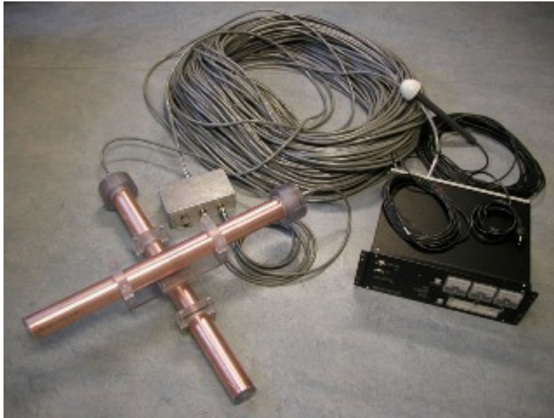
Figure 3.14: Image of the 2-Axis Search Coil Magnetometer: KHO website https://kho.unis.no/Instruments/SearchCoilmagn.html
