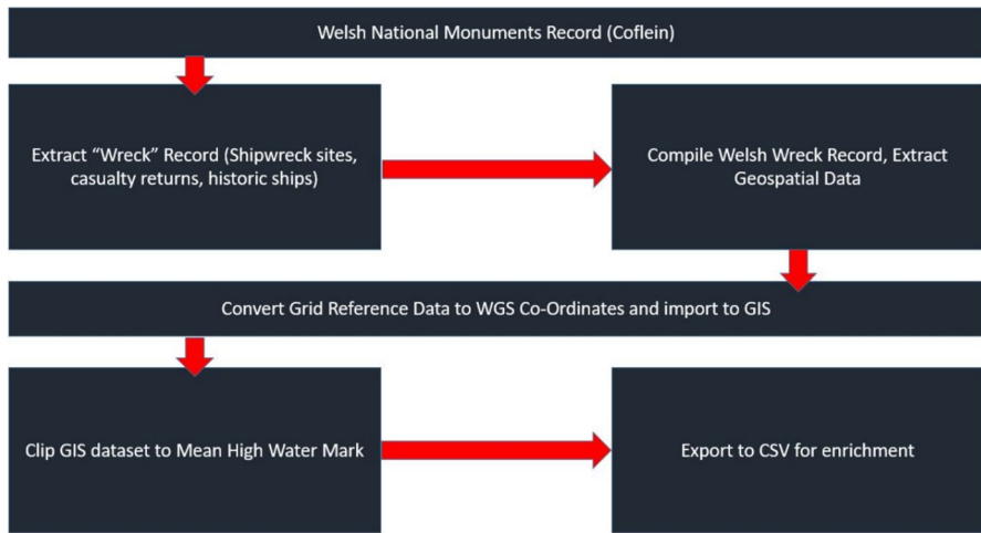
Fig. 2 An example of an extraction process for NMR data, this same pipeline can also be used to extract records from UKHO shapefiles (image by authors)
