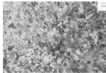
Etched metal structure beneath transparent coloured film on Cu-10Ni after 4 h impingement at 17 m s -1 .
