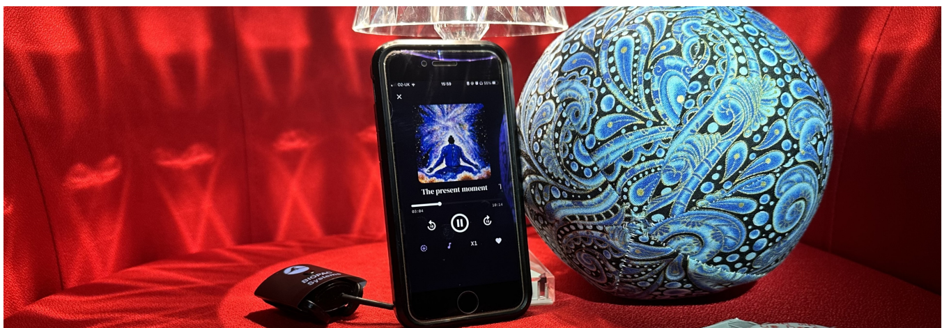
Figure 1: Experimental setup comprising the Digital Mental Health Intervention (DMHI), the shape-changing biofeedback physicalization called 'Ankor', and the Biopac Respiration Transducer.
