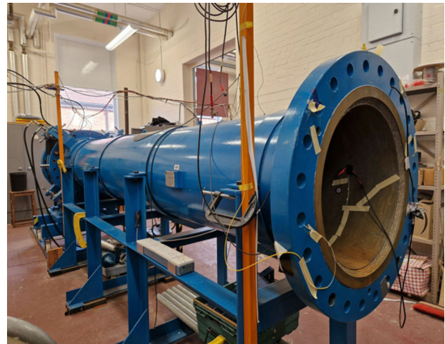
Fig. 4 Photograph of the shock tube at Cranfield University, UK, showing the full experimental arrangement and overall scale. The internal sensing fibre, secured to the inner tube wall with masking tape, is also visible
