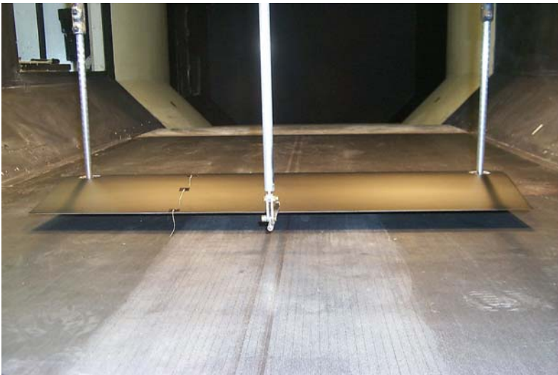
Figure 3: DMTU section in 2.1 x 1.7 m rolling road wind tunnel
