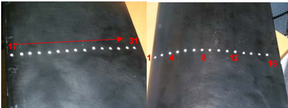
Figure 20: Location of Pressure Tappings on the DHMTU Lower (left) and Upper (right) surface
