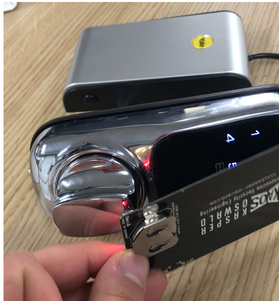
FIGURE 3.10: Chameleon device unlocking Yale Smart Lock
