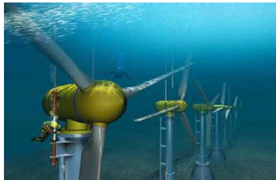
Fig. 1: A typical horizontal axis free stream marine current turbine, ( http://www.e-tidevannsenengi.com/ accessed 14/3/2008)
