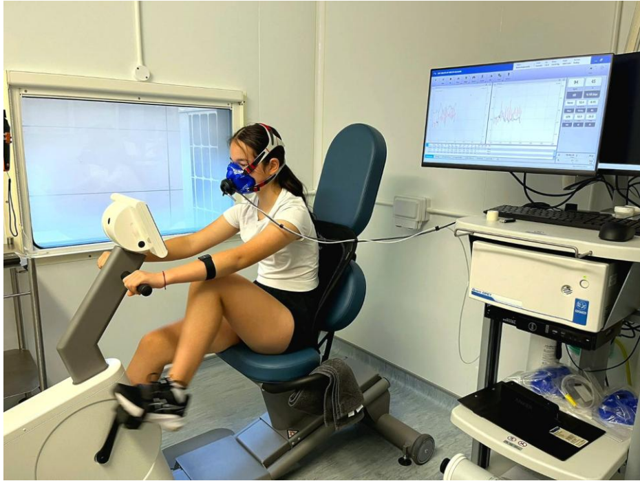
Figure 4-3. Participant performing exercise in the climate chamber with breath-by-breath analysis to calculate metabolic energy expenditure.
