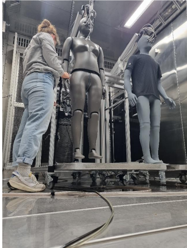
Figure 9-2. Male and female thermal manikins in the climate chamber.
