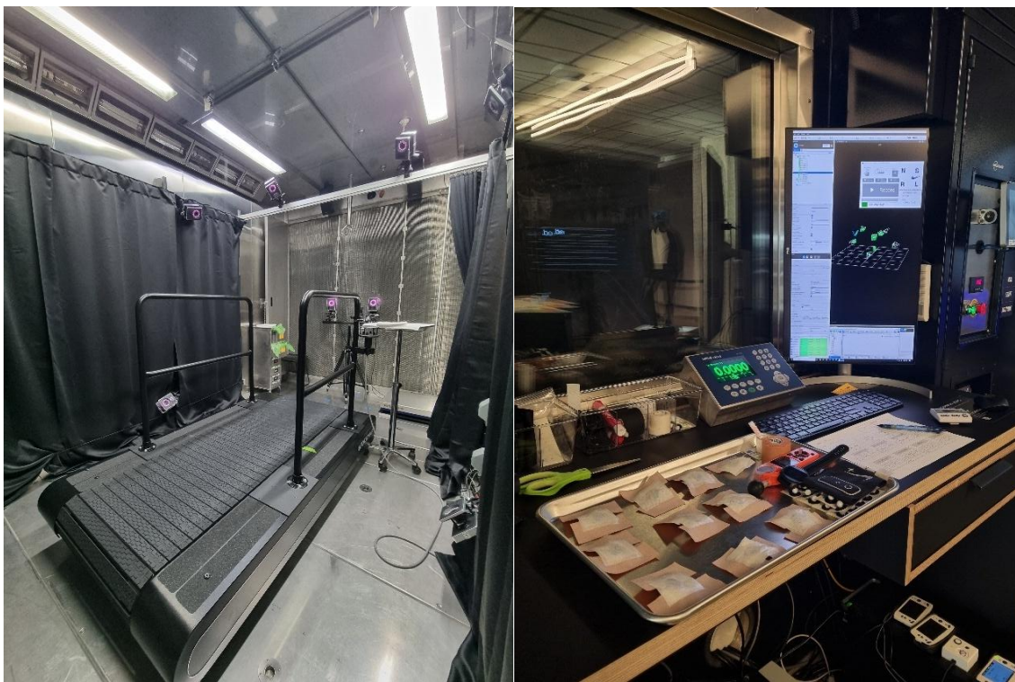
Figure 9-3. Climate chamber equipped with VICON motion capture.
