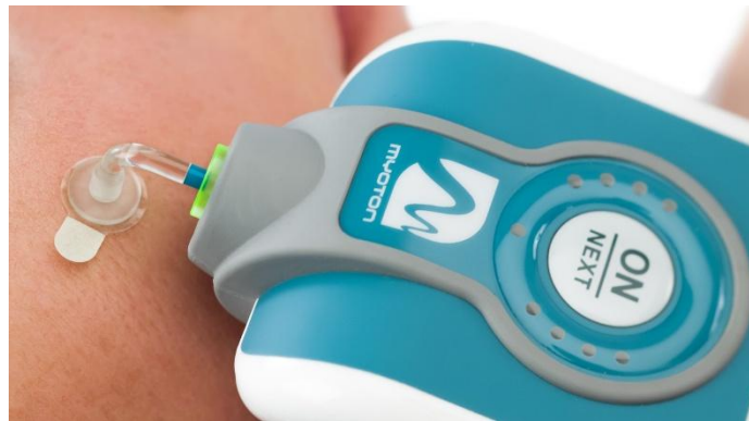
Figure 4-6. MyotonPRO device with J-shaped probe.
