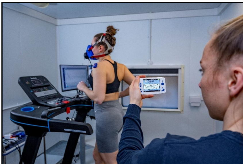
Figure 4-1. Core temperature reader device collecting data whilst the participant runs on a treadmill in the climate chamber.
