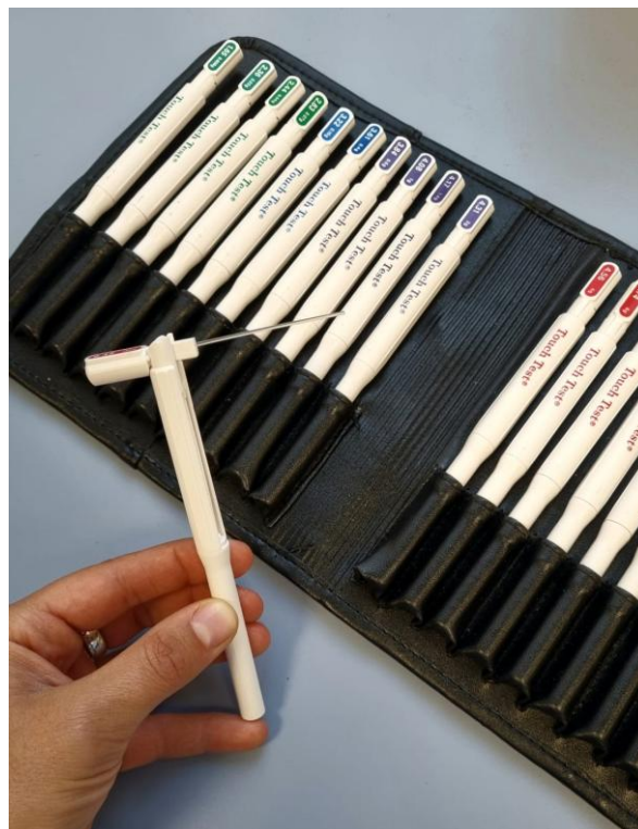
Figure 4-10. Von Frey monofilaments used to measure tactile thresholds
