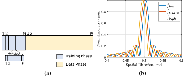
Figure 2. Frame structure utilized for wideband MU THz hybrid MIMO system using SC-FDE
