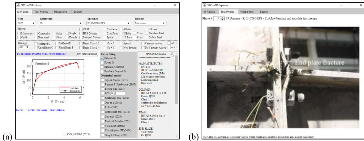
Fig. 2-24 Experimental database GUI: (a) digitised M-\theta data and bilinear fitting; (b) reported photo of damage and failure mode(s).
