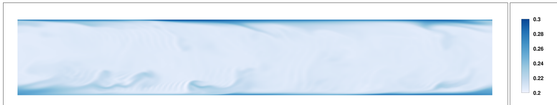
(e) Contour slice of \text{N}_2 mass fraction at z = 50\% . Colour bar ranges from 20\% to 30\% .
