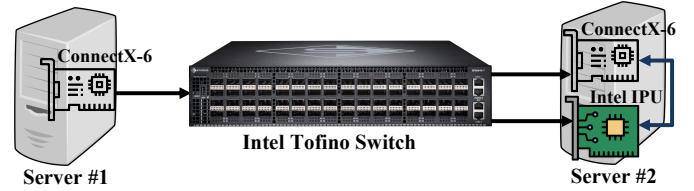
Figure 2: Testbed setup. The two servers are equipped with Mellanox ConnectX-6 NICs and are connected via an Intel Tofino switch. Fast-path ML inference runs on the Intel IPU in Server #2, where the NIC and IPU are also interconnected.
