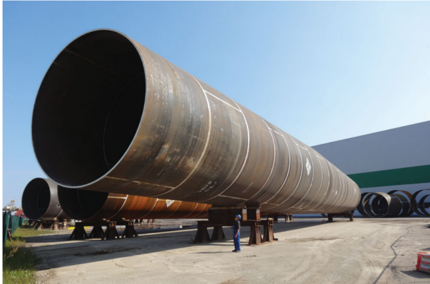
FIGURE 2.2: A 7.5 m diameter monopile foundation for an offshore wind turbine (Kallehave et al., 2015)
