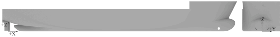
Fig. 1. The hull model of the case ship and the global coordinate system for CFD analysis.
