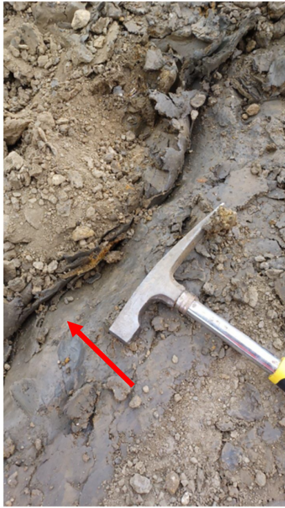
Fig. 5. An individual discontinuity surface at 0.6 m bgl in the Charmouth Mudstone Formation (Lias Group) near Ladbroke (LA), Warwickshire.
