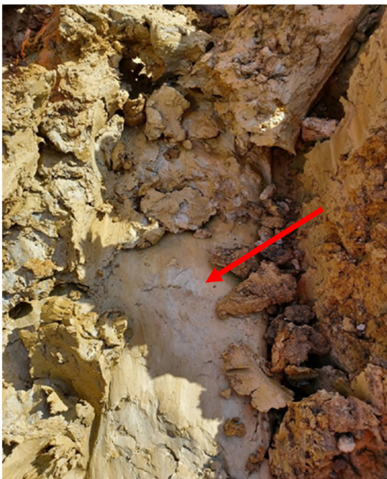
Fig. 8. Shallow dipping, undulose, closely spaced shears (Type 1) at 0.6 m below the original ground surface in orange to brown mottled grey silty clay of destructured Whitby Mudstone (Lias Group) near Brackley (BR), Northamptonshire.
