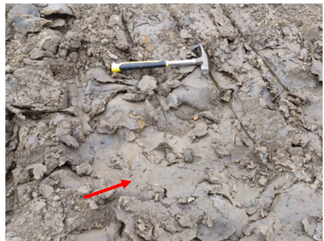
Fig. 4. Shears in the form of undulose pillow-like polished surfaces at c. 0.6 m bgl in the Charmouth Mudstone Formation (Lias Group) near Ladbroke (LA), Warwickshire. The hammer is 280 mm long.
