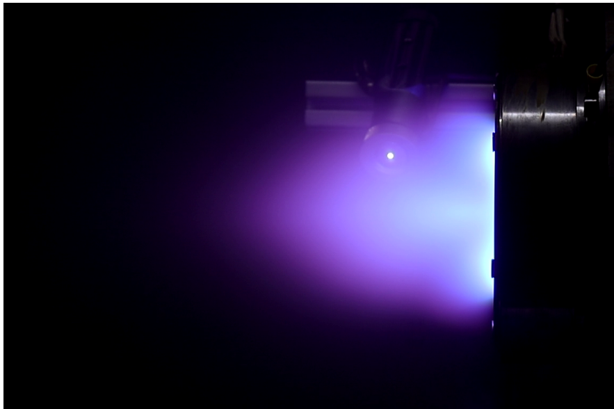
FIGURE 5.61: The TAL-1 configuration operating at approximately 1.3 kW on krypton within the large vacuum chamber facility at the University of Southampton.
