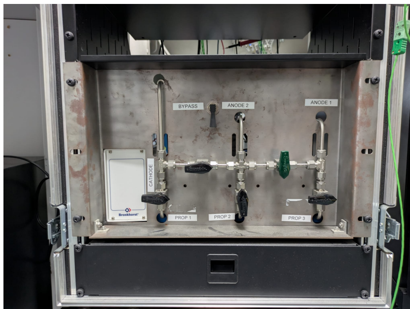
FIGURE 5.6: Photograph of the MAXPDS front control board as implemented for the SHARK-600V test campaign.
