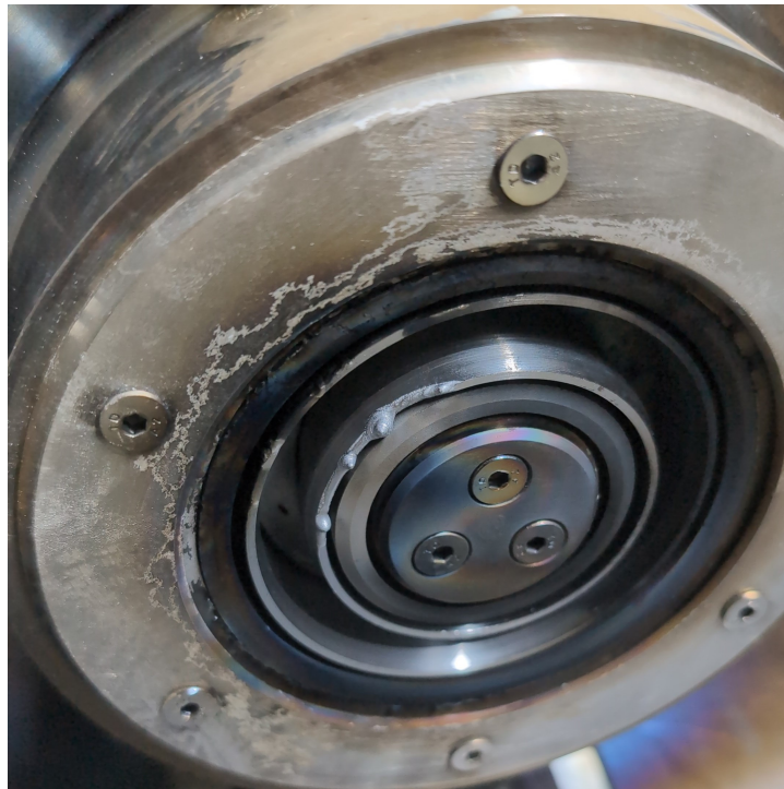
FIGURE 5.67: The “TAL+1” metallic anode after high thermal load conditions. The image shows the post-operation state and the resultant structural failure after melting, observed once the chamber was returned to atmosphere.
